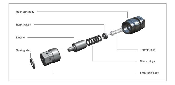
The Thermal and Pressure Relief Device (TPRD) 016280-K is used to secure gas storage tanks in the event of a fire by ensuring rapid and spatially targeted degassing at elevated temperatures whilst preventing the tanks from bursting.
