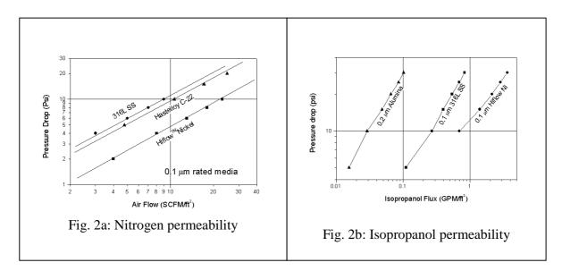
The sintered metal microfiltration media are designed to be used in cross flow filters when filtering liquids. The Hiflow<sup>TM</sup> Nickel in slightly modified form is also used for semiconductor gas filtration with an efficiency of 9 LRV (log reduction value).
